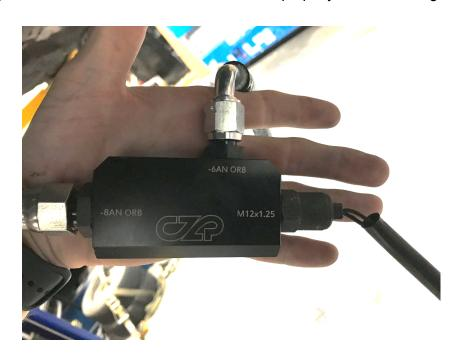
6. Now that the manifold block is fully assembled, you can go ahead and connect each of the lines to their respective fittings on the manifold block and tighten them down snugly. The -6AN 90 degree line on the top of the block should be angled towards the rear (away from the CZP logo and labels).
